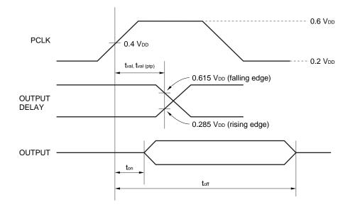
Figure 7-3. PCI Output Timing
