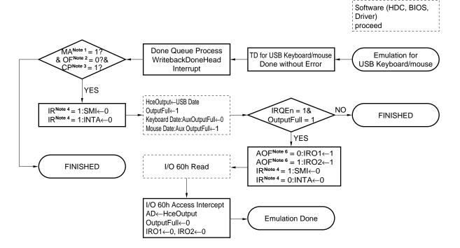
Figure 3-18. Input Emulation Flowchart for USB Keyboard/Mouse
