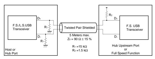
Figure 3-2. Full Speed Device Cable and Resistor Connections
