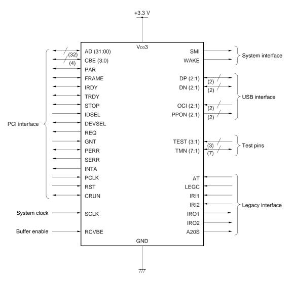
Figure 1-2. Pin Configuration
