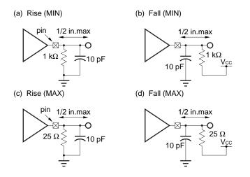
2. The measurement conditions for the PCI output slew rate are the same as (a) and (b) above.
