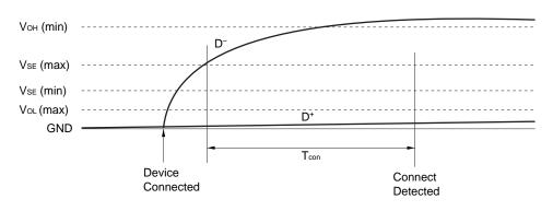
Figure 7-9. USB Low Speed Device Connect Detection
