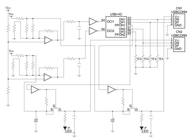
Figure 8-1. Circuit Example of USB Interface Block
