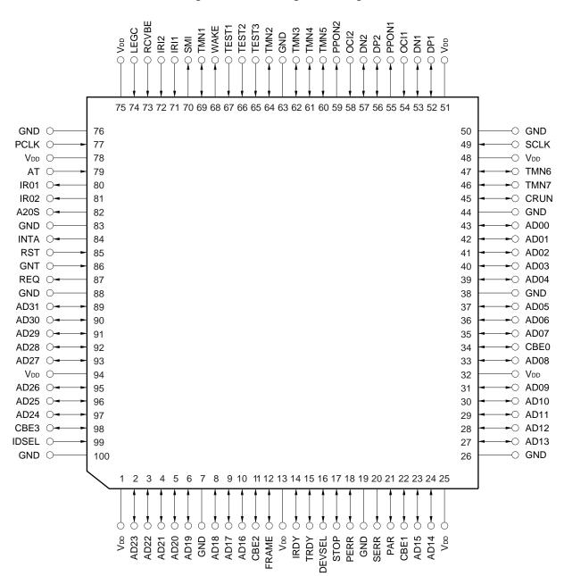
Figure 1-3. Pin Configuration Diagram
