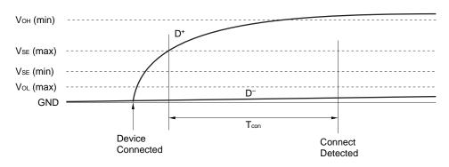
Figure 7-8. USB Full Speed Device Connect Detection
